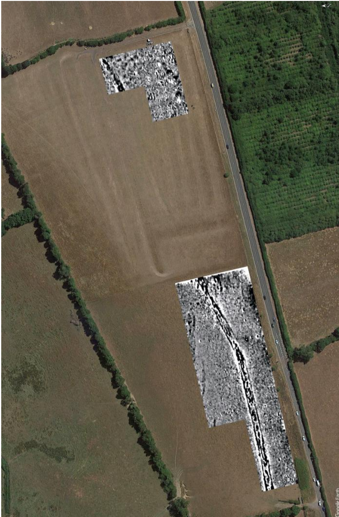
Fig (08) Magnetometer Results at two locations East and West showing clear indications of a road way.
